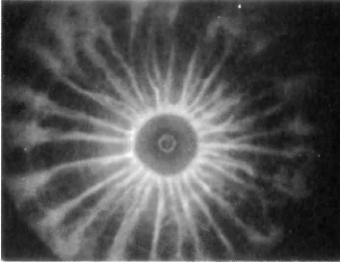
Fig. 6.13a. As the sheath carrying the inward-moving current forms, pairs of vortex filaments are generated.
