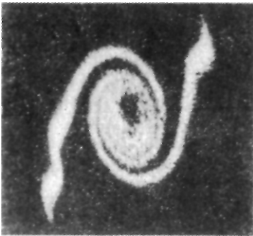
Fig. 1.12. Spiral filaments of current and glowing plasma, a few millimeters across, are formed in the lab, resembling the mighty spiral galaxies of space (A. Peratt).
